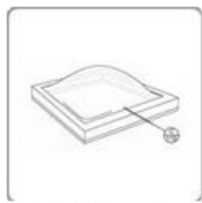
Curb Mounted Skylight
